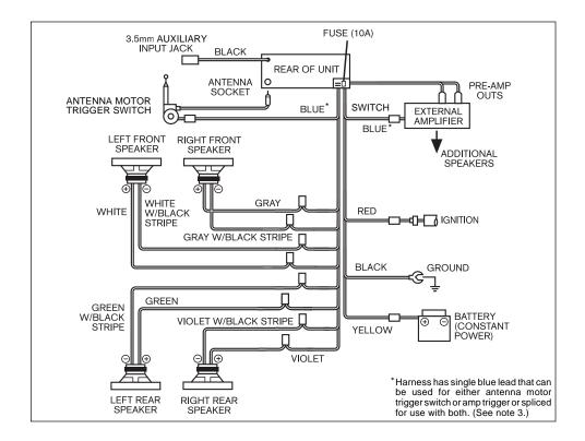
and connect the speaker(s) directly to the amplifier.
